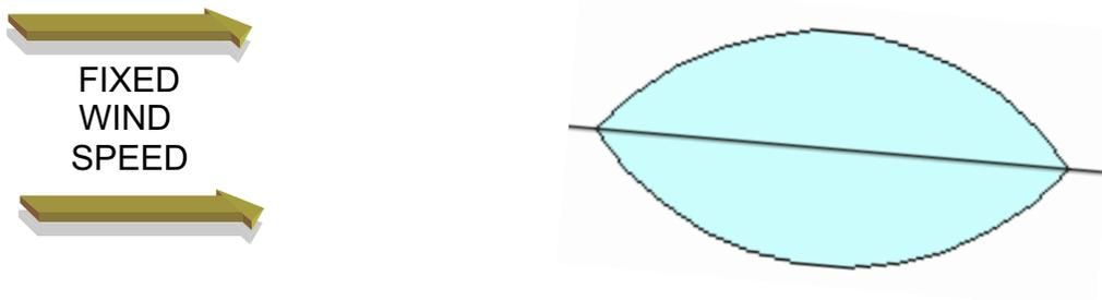
A slight rounding of the nose will stabilize the object and make it less susceptible to this behavior at the expense of some increase in resistance.
